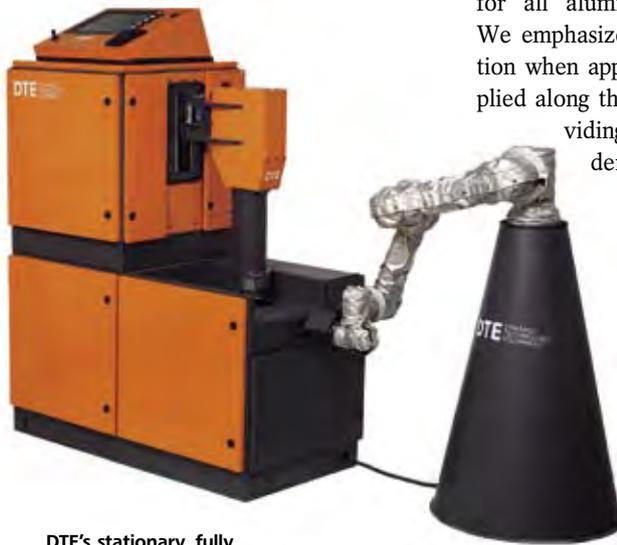
DTE’s stationary, fully automatic, elemental analyzer EA-2500 to measure chemical composition analysis from furnaces and launders, directly from the equipment (DTE EA-2000) or taking samples from them (DTE EA-2500)
