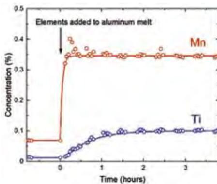
The melting dynamic of the elements added to the aluminum melt for a given furnace is the basis for the alloying optimization system's model, optimizing the alloying process by defining the loading volume, sequence, and order
