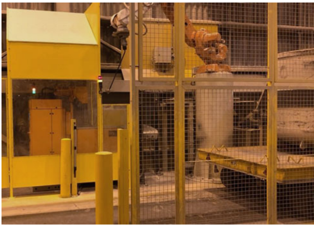
Fig. 2 Robot feeds sample of liquid Al to LIBS analyzer
