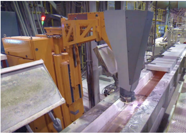
Fig. 1 LIBS analysis directly in casting launder
