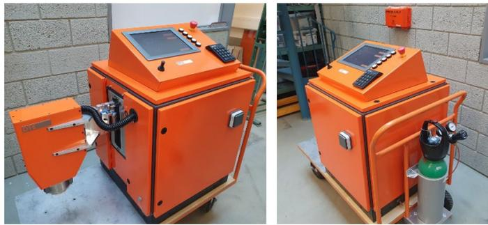
Figure 1. Portable liquid metal analyzer.
