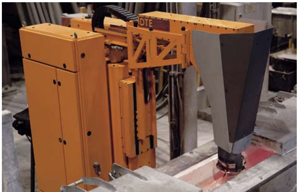
DTE's Stationary Elemental Analyzer EA-2000 performing chemical composition analysis at the launder
