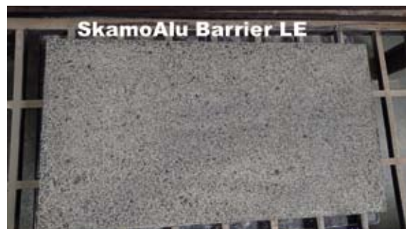
SkamoAlu Barrier LE is an insulating barrier board with a density of 1,400 kg/m 3
