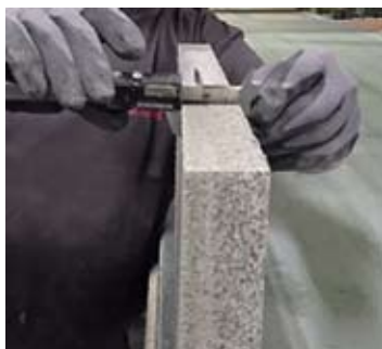
SkamoAlu Barrier LE is an insulating barrier board with a density of 1,400 kg/m 3
